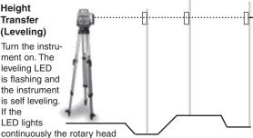
starts and the laser beam will be turned on. Attach the PLS HLD 1000 Detector at this reference point on a rod and move this height to zero. Now the respective difference in levels to the reference height can be measured on the ground. It is useful to use a flexible rod to measure positive and negative values simply.
